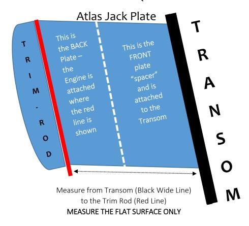
4" and 6" Atlas Jack Plates are built in one part only. There will be **NO** "spacer" plate as shown in the picture above.
